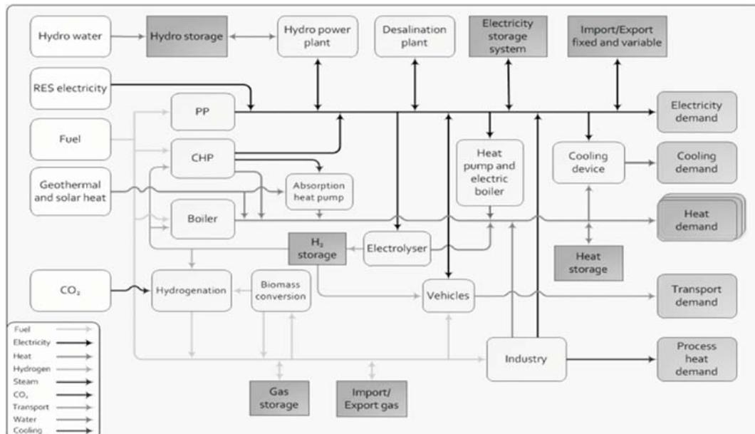
Figure 1. EnergyPLAN System Diagram – Version 11.2 - November 6, 2013
