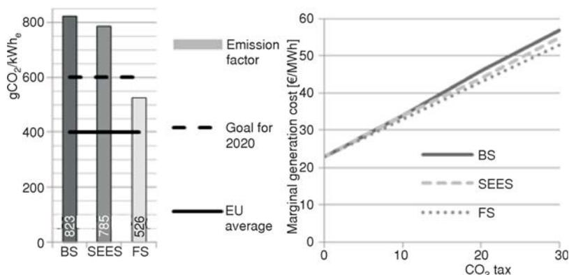
**Figure 3. Emission intensity of Serbian electricity sector in comparison to EU (left); sensitivity analysis of TPP marginal generation costs under CO<sub>2</sub> prices change (right)**
